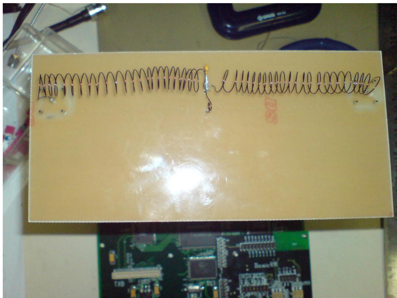
Figure A.4: Bandpass filter construction
