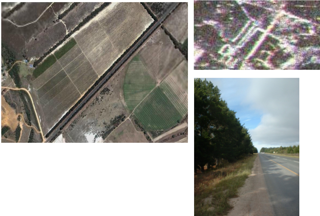
Figure 5.10: Road lined by trees as seen by optical photo (left) and SASAR sensor (top right). The Road appears as a bright line diagonally across the SASAR image.
