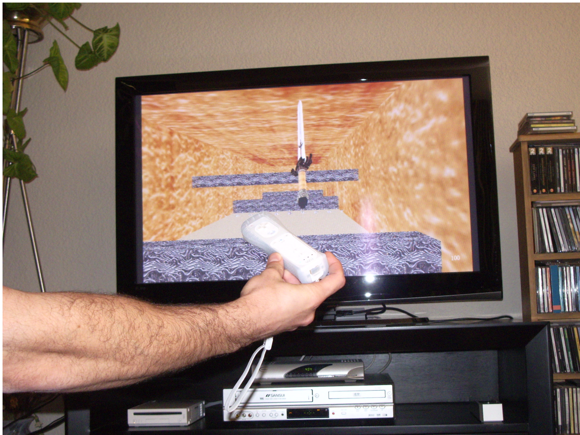
Figure 5.10: Photograph of item manipulation with a yaw rotation which cannot be measured and, hence, isn't depicted in the in-game object
