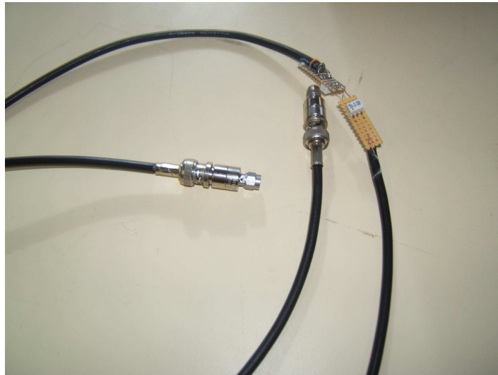
Figure 4.2: Transformers connected back-to-back and coaxial cable.
