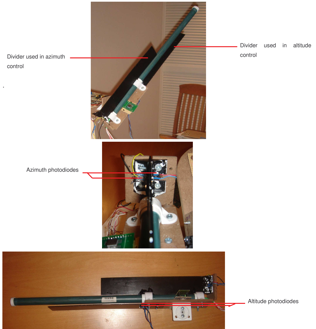
Figure 14: Photodiode system mechanics
