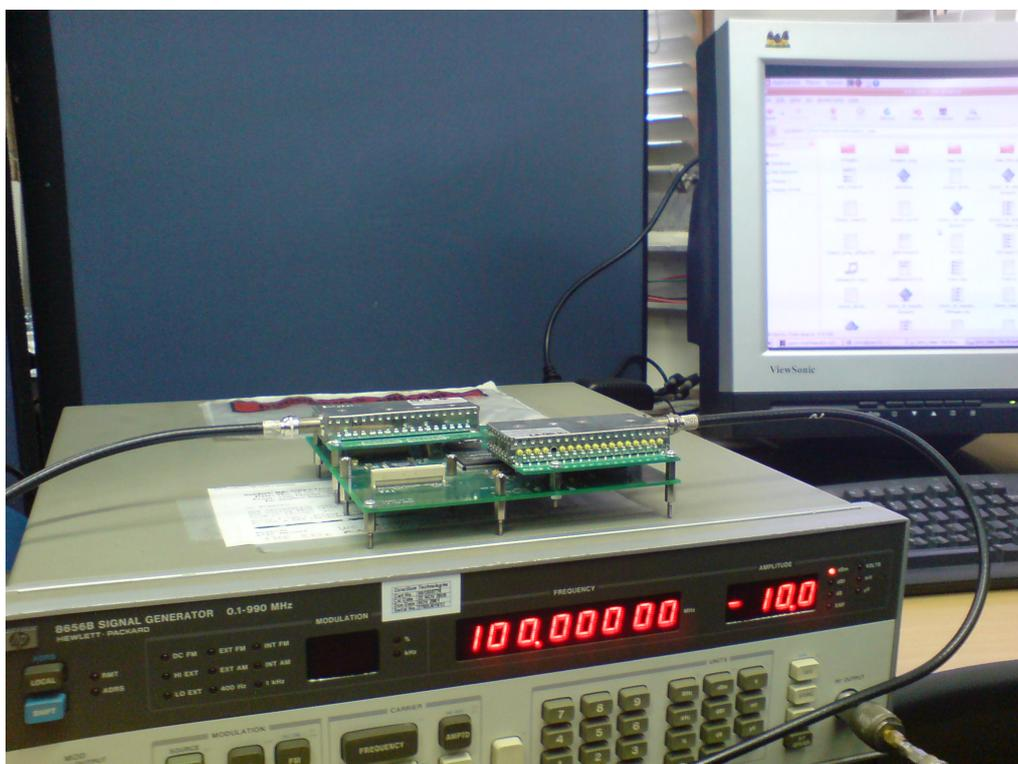
Figure C.3: USRP and signal generator
