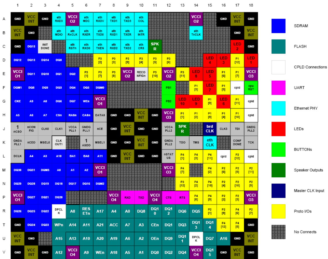
Figure 5.11: Cyclone 1C12 Functional Pin-out, courtesy of [13]
