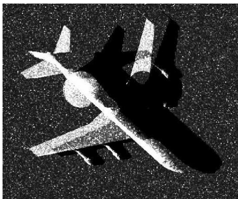
Figure 1.1: Simulated SAR image of E-3 sentry aircraft, created by SARviz (from [1])
