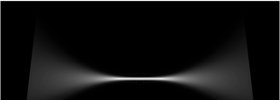
Figure 3.5: The magnitude of the signal in the range-Doppler domain after the range curvature correction operation (Simulation A). Only the first 100 of the 528 slant range bins are displayed (range increases vertically). The full 250 Hz sampling bandwidth is represented by the horizontal extent of the image.
