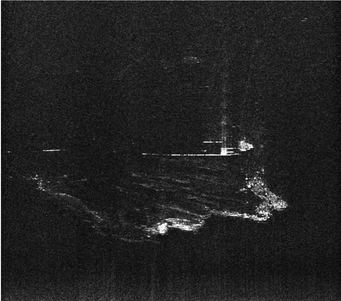
Figure 6.5: SASAR VHF HH image of the Cape Agulhas area. The image extent is 13 km on a side with slant range increasing vertically. 25 m range resolution, LMS adaptive interference suppression, range compression, 22 m nominal azimuth resolution, 4 looks (2.5 independent), range compression.
