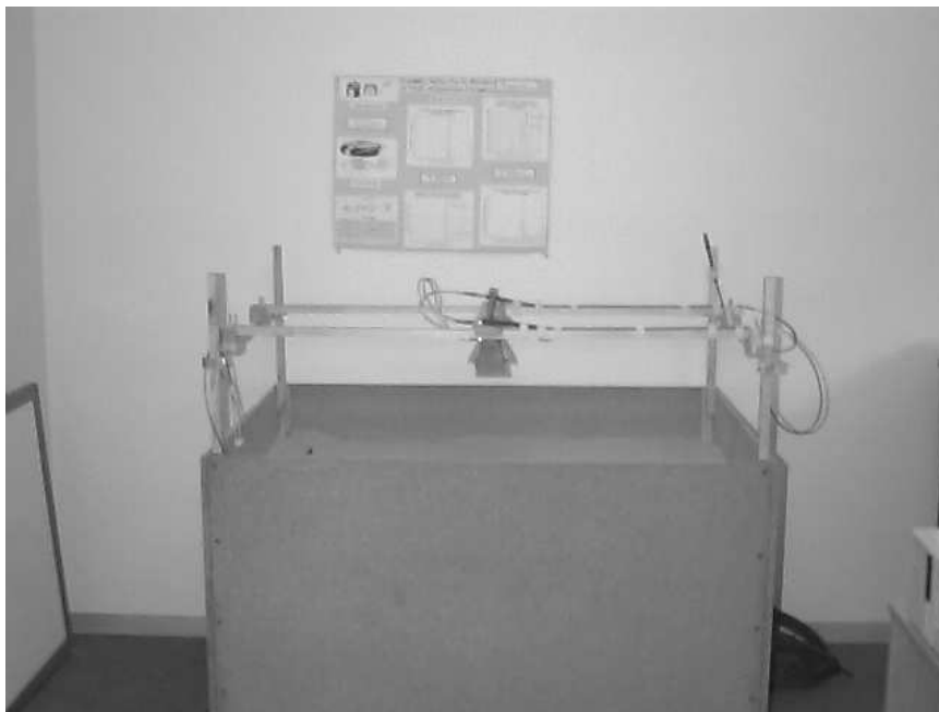
Figure 3.16: Photograph of the antenna setup for the polarimetric measurements.
