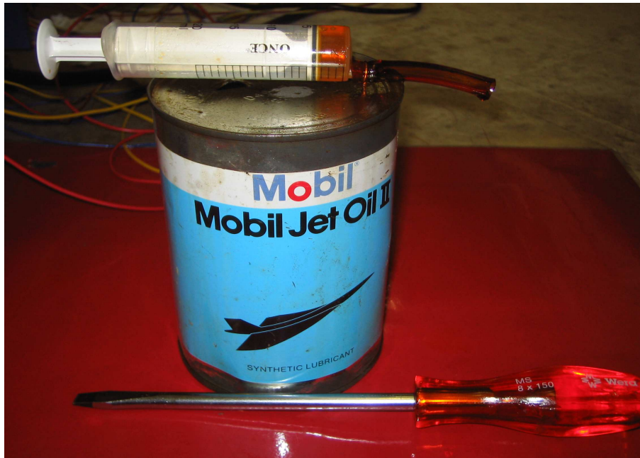
Figure 4.6: Tools used to re-fill the gearbox sump
