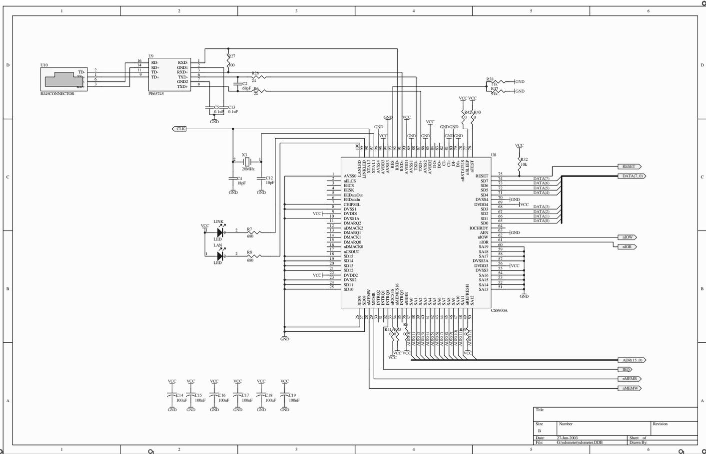
Figure 8.2: Ethernet controller schematic
