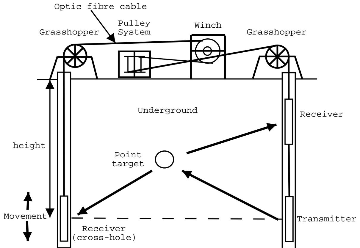
Figure 2.2: Geometry of bore-hole survey (with reference to [20])
