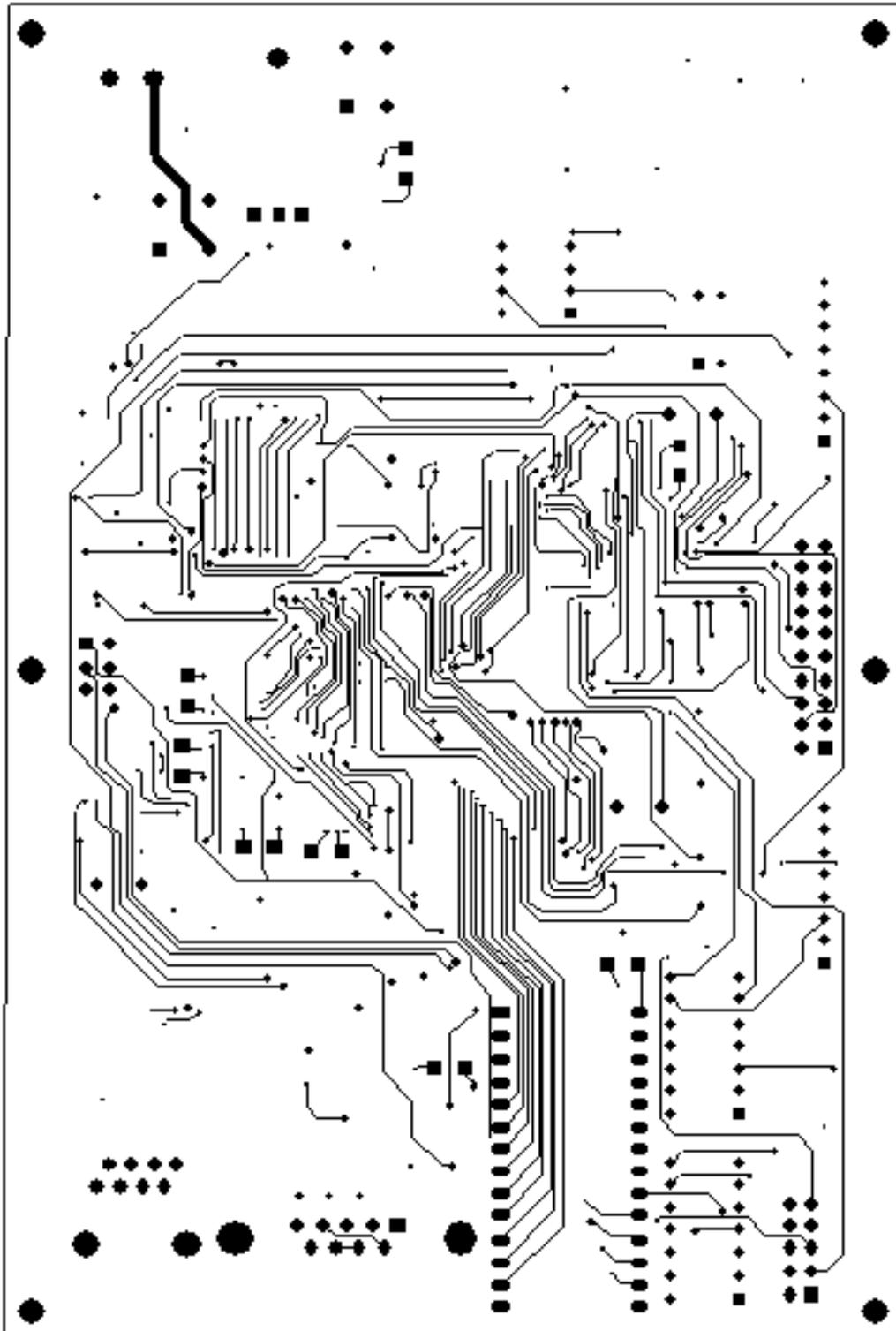
Figure 8.6: Bottom layer for PCB
