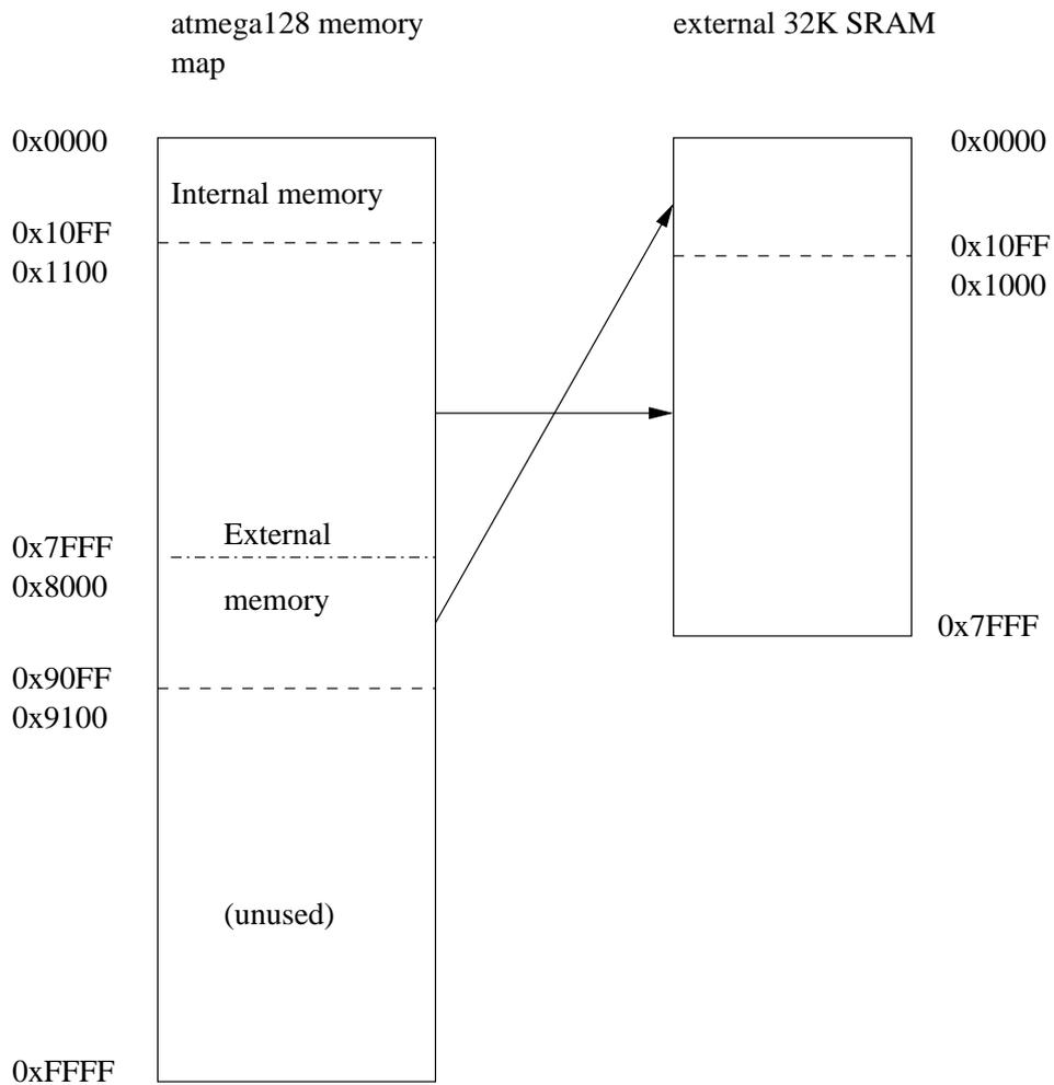
Figure 3.7: Atmega128 memory map(with reference to [10])
