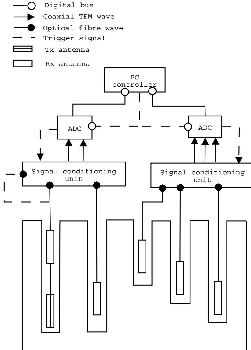
Figure 2.1: Block diagram of BHR (with reference to [20])
