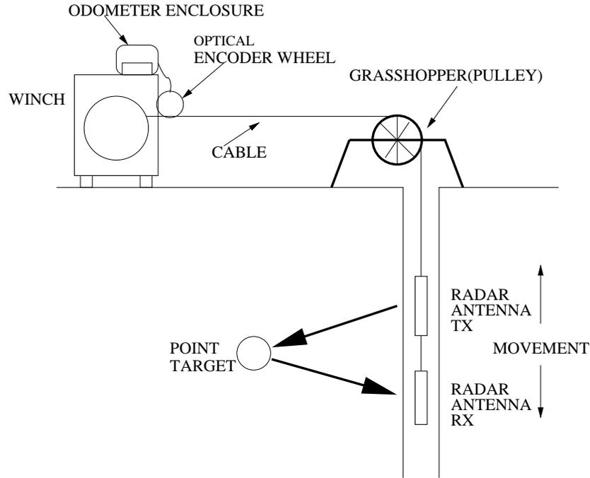
Figure 1.2: Radar deployed in bore-hole
