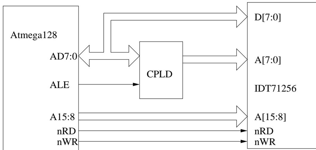
Figure 3.6: Atmega128 interface with SRAM
