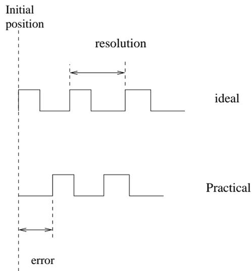
Figure 2.5: actual position of slot on disk of encoder
