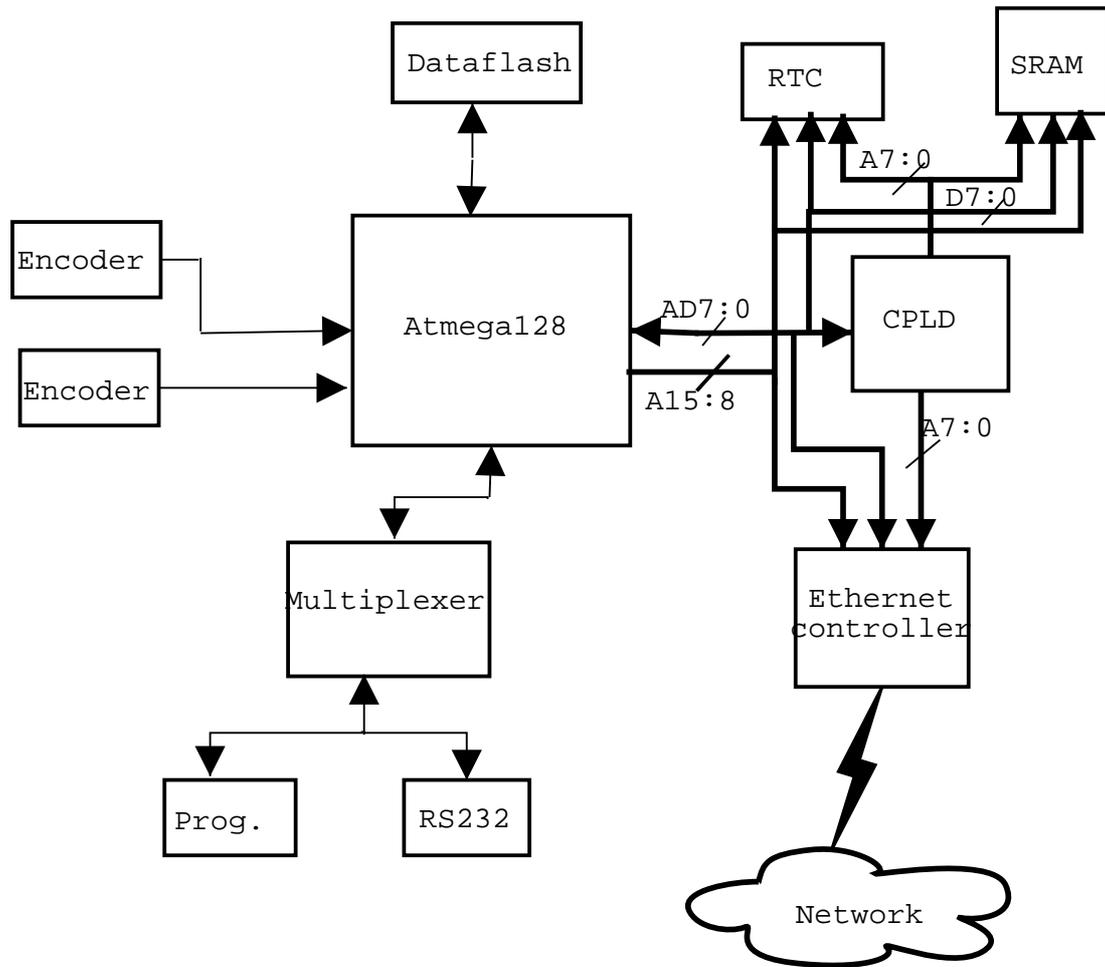
Figure 3.3: Block diagram of Odometer
