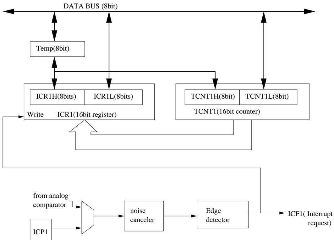
Figure 3.5: Input capture unit (with reference to [10])
