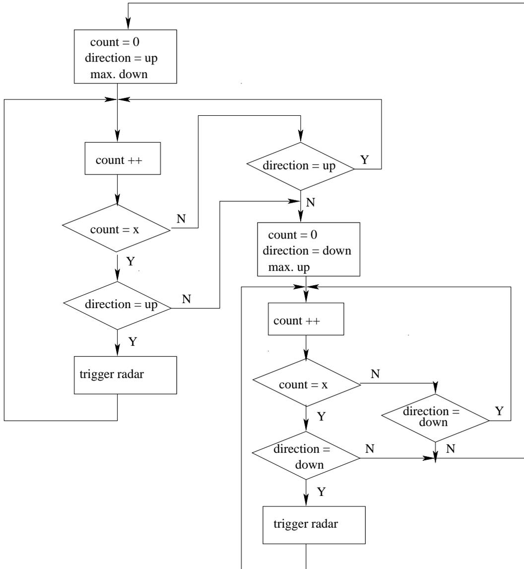
Figure 4.2: Flow chart for non timestamped data
