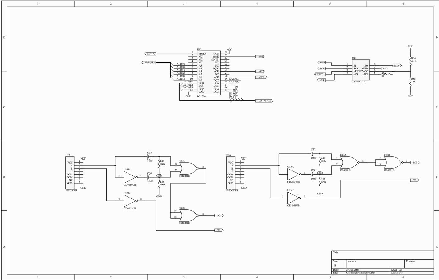
Figure 8.3: Encoder, RTC and Dataflash schematic
