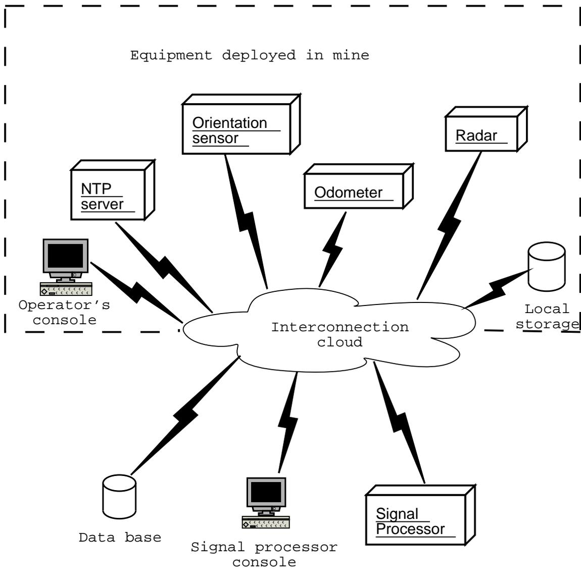
Figure 1.3: Setup of Geophysical Recording and Processing system
