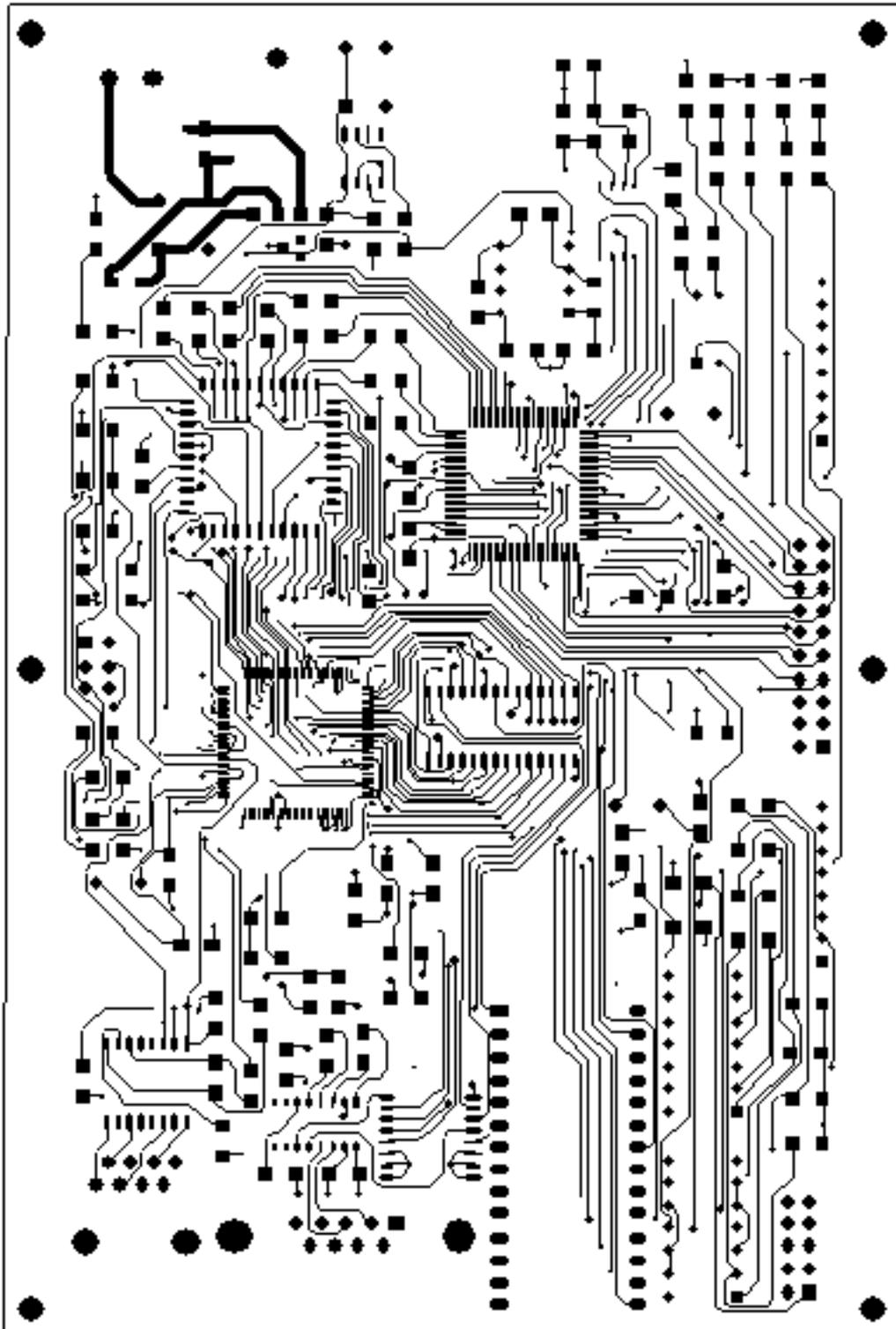
Figure 8.5: Top layer for PCB
