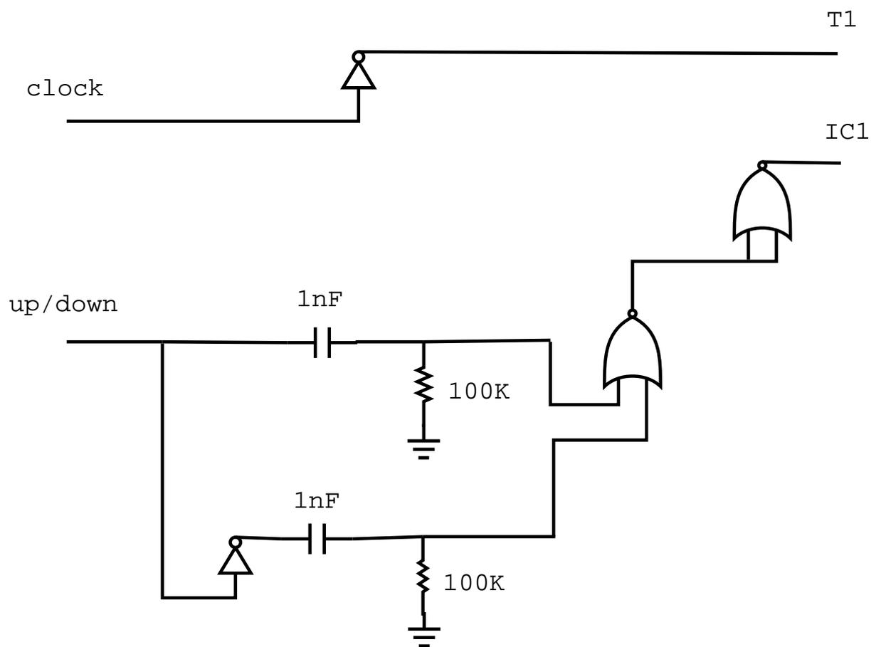
Figure 8.9: Circuit diagram of encoder to microcontroller interface
