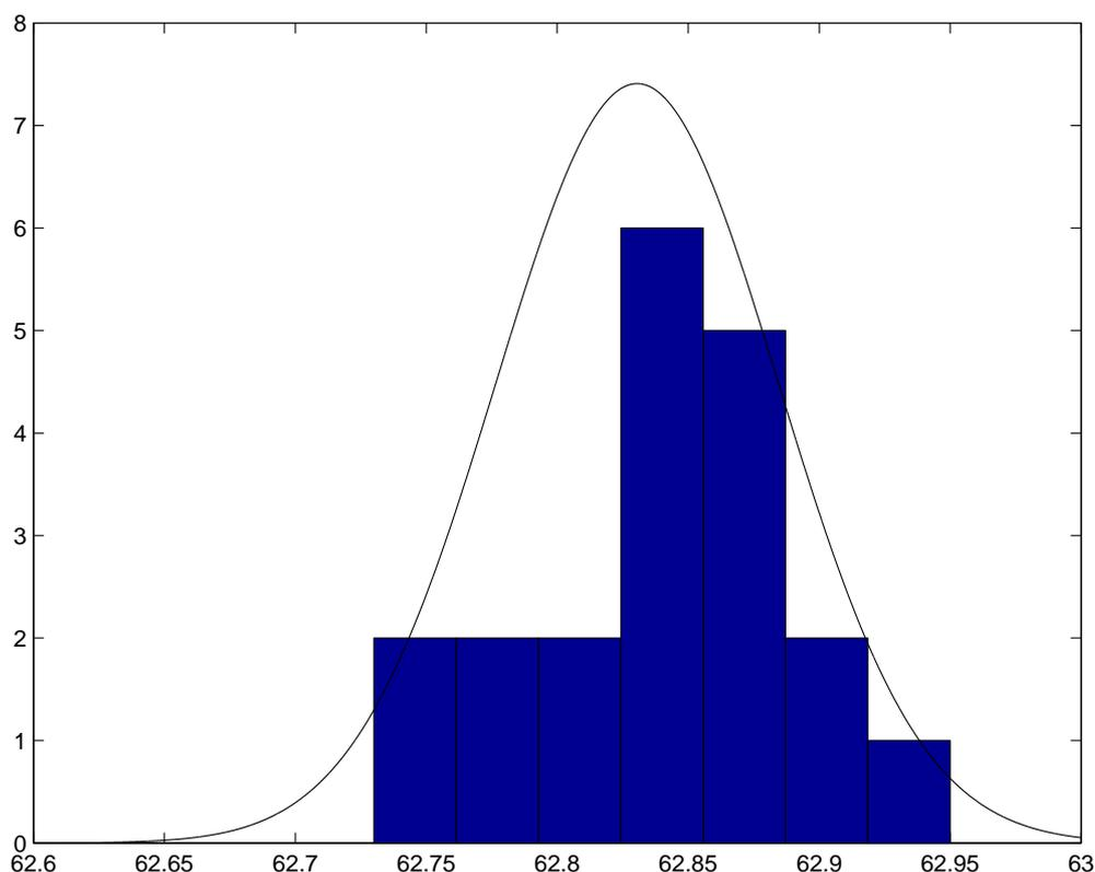
Figure 5.2: Gaussian distribution and histogram of encoder wheel circumference
