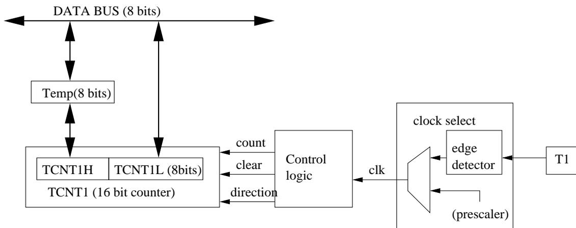
Figure 3.4: Counter unit (with reference to [10])
