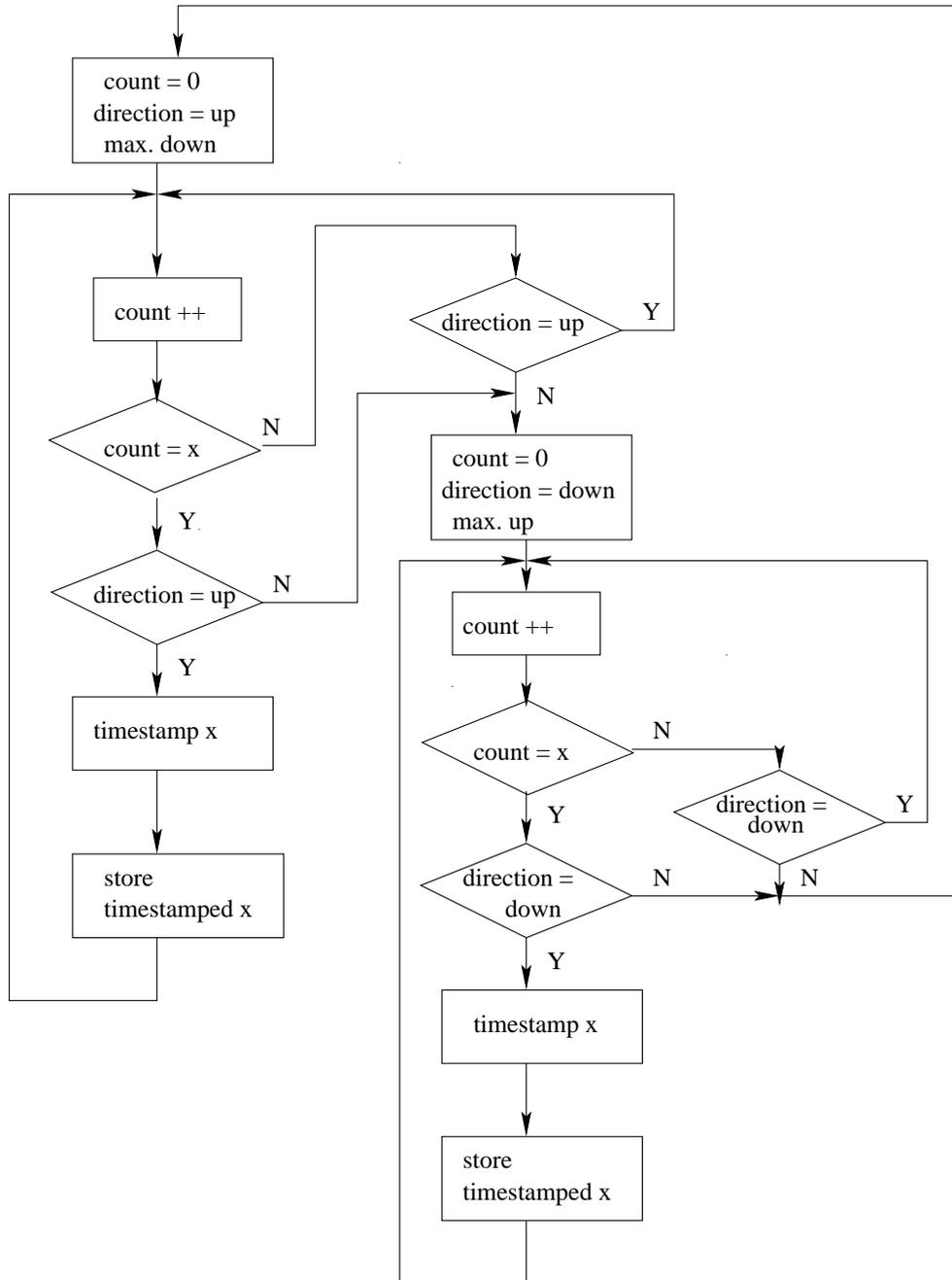
Figure 4.1: Flow chart for time-stamping the data
