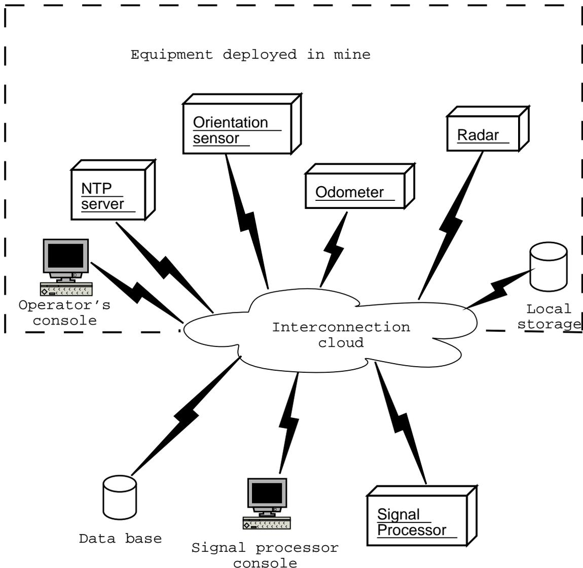
Figure 2.3: Geophysical recording and processing system (with reference to [17])
