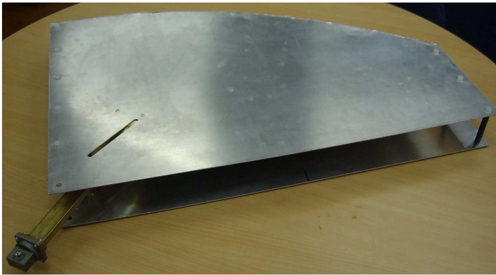
Figure 3.9: Top View of Fully Constructed Antenna
