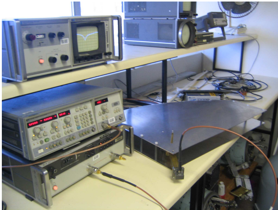
Figure 4.3: Experimental Setup for RL Measurement
