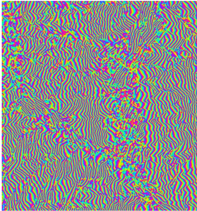
(a) Example of fringe rate due to a 160m baseline
