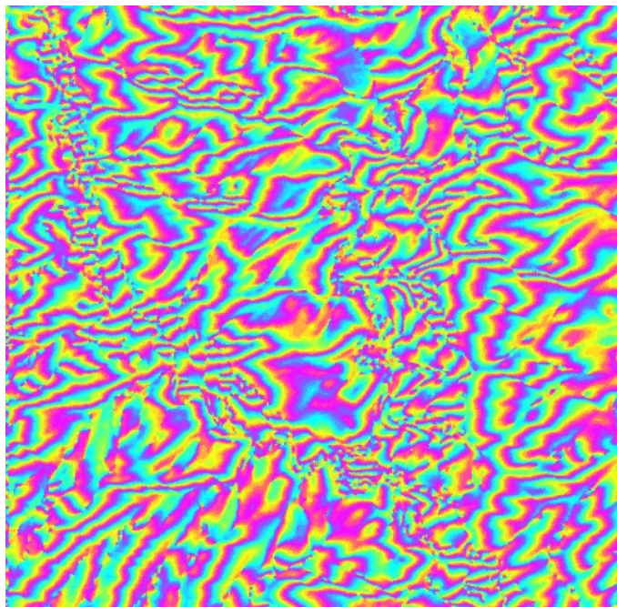
(b) Interferogram (92m baseline) flattened by subtraction of average fringe rate.
