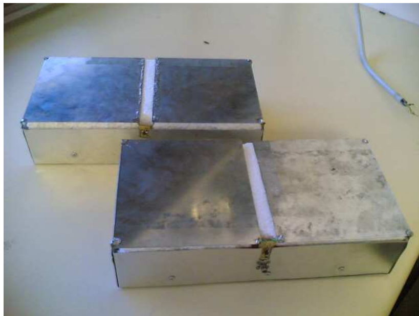
Figure 5.3: Photograph of the antennas and S11 sand box testing arrangement with Agilent E5062A network analyser
