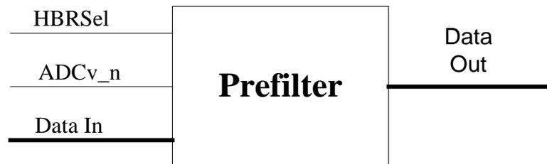
Figure 14: Top Level Block Diagram of the Prefilter
