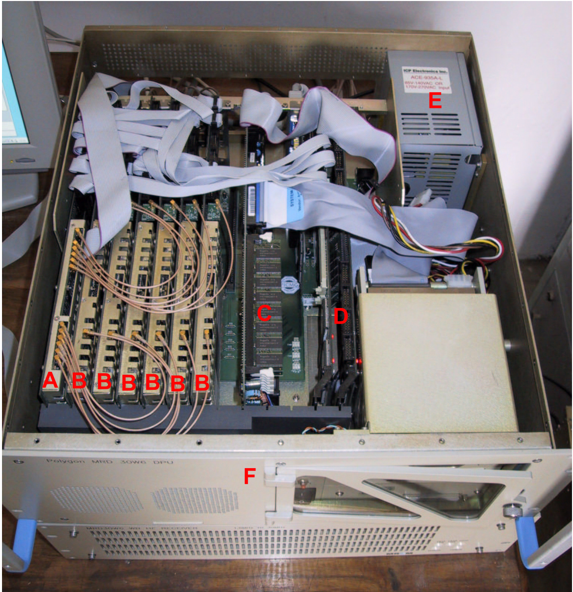
Figure D.2: 6-Channel wideband digital receiver.
