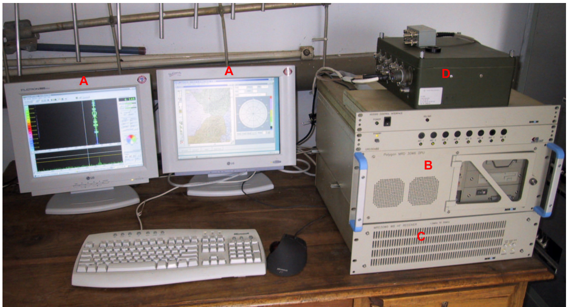
Figure D.1: 6-Antenna wideband receiver incorporating the digital receiver.
