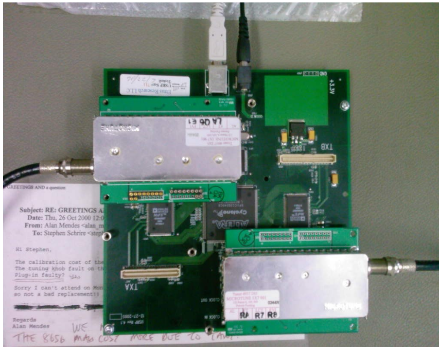
Figure 1.4: USRP with two TVRx boards, reference channel and target channel
