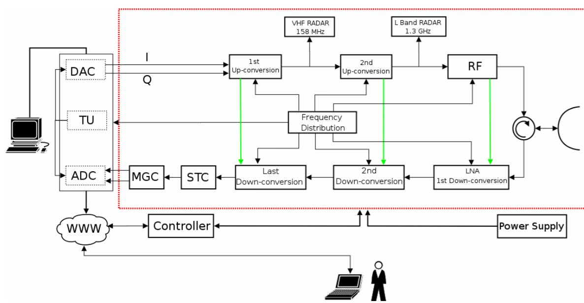
The SASAR II system consists of a three stage up-conversion transmitter with intermediate frequencies at 158 MHz, and 1.3 GHz. The input to the transmitter is generated by the digital to analogue converter. For the purposes of this dissertation the testing was restricted to low power loop back testing.
