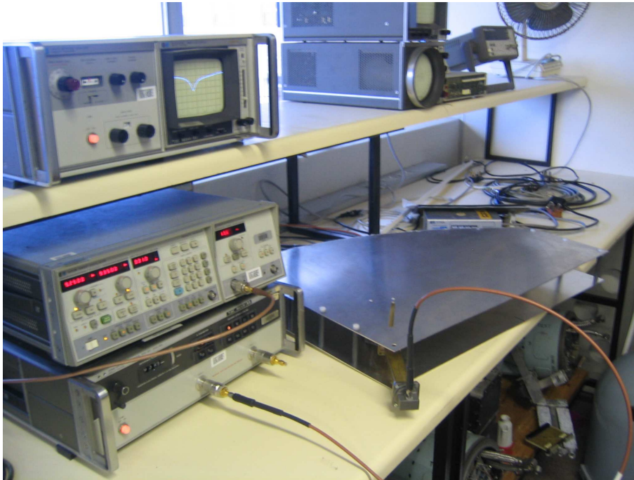
Figure 4.3: Experimental Setup for RL Measurement
