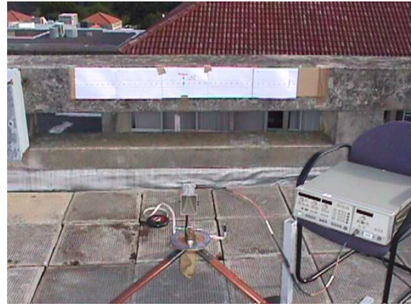
Figure 13: Receive horn with the 'dotted' background chart
