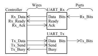
The wire type is employed to connect an output of one logic element in a circuit to an input of another logic element. The following are examples of scalar wire declarations.
