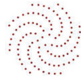
Illustration of how just a few points arranged into a Vogel spiral looks
